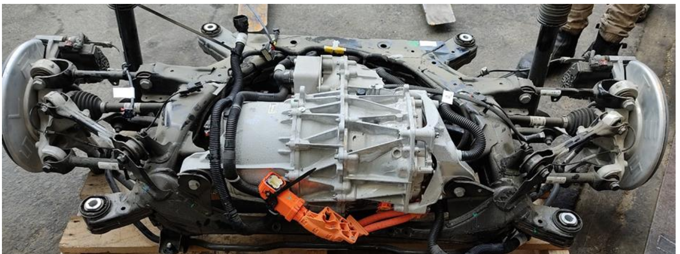
197hp 2021 Tesla Model3 rear axle on subframe
