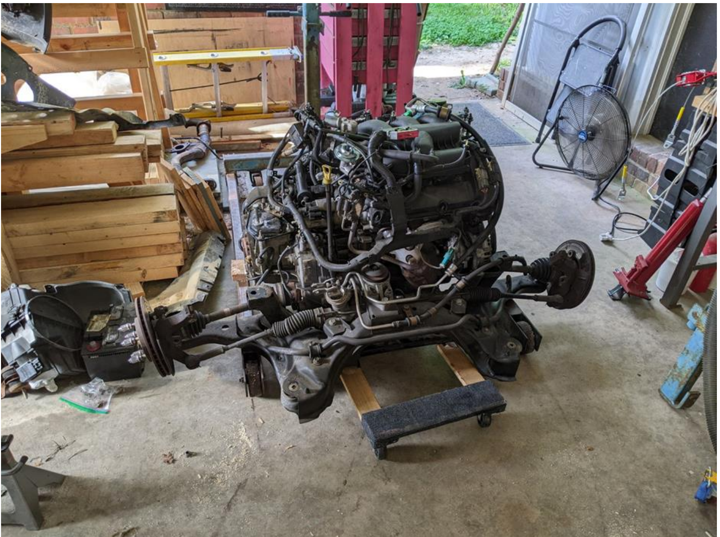
Mazda Tribute V6 3.0L 220hp, front axle on subframe. Picture source internet.
